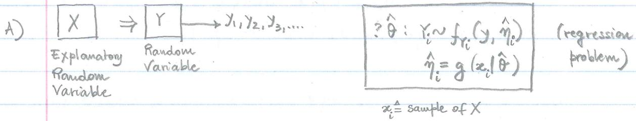
In this problem, we assume that the vector of parameters  $\eta_i$  is a function of the value of RV  $X \Rightarrow$  We must estimate the parameter vector  $\hat{\theta}$  that uniquely defines the function between  $x_i$  and  $\eta_i \forall i$ .
