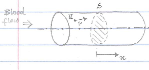
We would like to determine the quantity of blood  $Q$  that flows through the cross-section  $S$  per unit time (i.e., flux through  $S$ )
