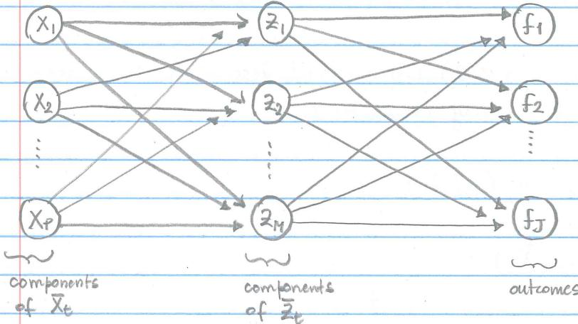
The solution is obtained by following a feed-forward network, in which one layer of variables (i.e.,  $\bar{z}_t$ ) is not directly observed, i.e., it is HIDDEN
